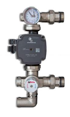
The control pack has <sup>3</sup>/<sub>4</sub>" flow and return connections with the flow being the top connection and the return being the bottom.
